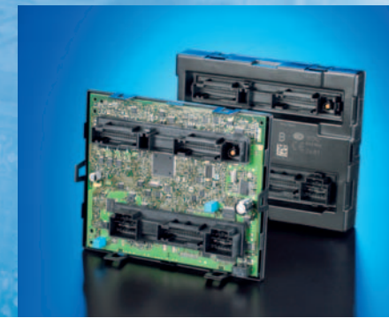
Central control unit for lighting, access, radio remote control, comfort and power
